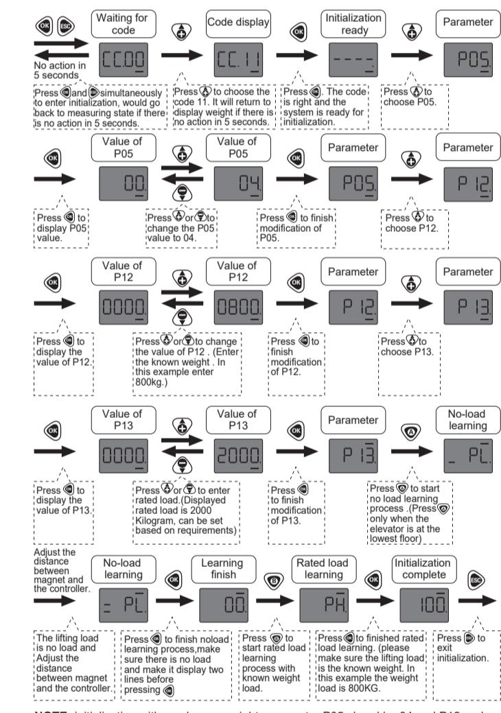
NOTE: initialization with any known weight, parameter P05 should be 04 and P12 and P13 should also be modified. The equipment should lift known weight during rated load learning period. input rated load value to P13. Press OK to switch display in percentage or in weight.
