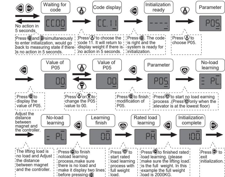
NOTE: initialization with full weight , P05 should be 00. The equipment should lift rated load. Input rated load value to P13, press OK to switch display in percentage or in weight.
