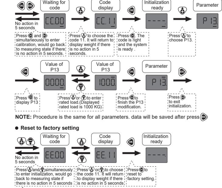
NOTE: Procedure is the same for all parameters. data will be saved after press OK.
