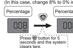
NOTE: before clearing tare, please make sure that the equipment has no load, good for both percentage and weight displays.
